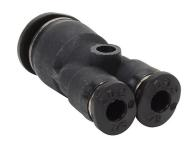
NITRA pneumatic push-to-connect fitting, union Y reducer, thermoplastic (PBT) body, (1) 1/4in push-to-connect to (2) 1/8in push-to-connect. Package of 5.
