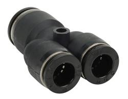
NITRA pneumatic push-to-connect fitting, union Y reducer, thermoplastic (PBT) body, (1) 1/2in push-to-connect to (2) 3/8in push-to-connect. Package of 5.
