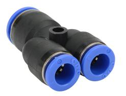
NITRA pneumatic push-to-connect fitting, union Y reducer, thermoplastic (PBT) body, (1) 10mm push-to-connect to (2) 5/16in (8mm) push-to-connect. Package of 5.
