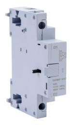
WEG Electric field installable undervoltage trip, right side mount, 400-415 VAC (50Hz)/480 VAC (60Hz) sensing range, screw terminals. For use with MPW40 and MPW80 series manual motor protectors.
