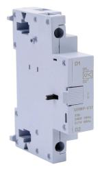
WEG Electric field installable undervoltage trip, right side mount, 230-240 VAC (50Hz)/240-277 VAC (60Hz) sensing range, screw terminals. For use with MPW40 and MPW80 series manual motor protectors.
