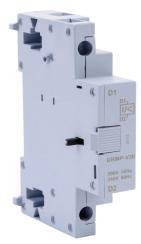
WEG Electric field installable undervoltage trip, right side mount, 208 VAC (50Hz)/240 VAC (60Hz) sensing range, screw terminals. For use with MPW40 and MPW80 series manual motor protectors.
