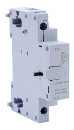
WEG Electric field installable undervoltage trip, right side mount, 110 VAC (50Hz)/120 VAC (60Hz) sensing range, screw terminals. For use with MPW40 and MPW80 series manual motor protectors.
