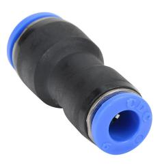
NITRA pneumatic push-to-connect fitting, union straight reducer, thermoplastic (PBT) body, (1) 5/16in (8mm) push-to-connect to (1) 6mm push-to-connect. Package of 5.
