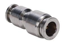
NITRA pneumatic push-to-connect fitting, union straight reducer, 316 stainless steel body, (1) 5/16in (8mm) push-to-connect to (1) 6mm push-to-connect.
