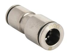
NITRA pneumatic push-to-connect fitting, union straight reducer, nickel-plated brass body, (1) 5/16in (8mm) push-to-connect to (1) 6mm push-to-connect. Package of 5.
