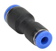
NITRA pneumatic push-to-connect fitting, union straight reducer, thermoplastic (PBT) body, (1) 6mm push-to-connect to (1) 5/32in (4mm) push-to-connect. Package of 5.
