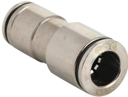
NITRA pneumatic push-to-connect fitting, union straight reducer, nickel-plated brass body, (1) 5/16in (8mm) push-to-connect to (1) 1/4in push-to-connect. Package of 5.
