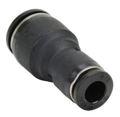
NITRA pneumatic push-to-connect fitting, union straight reducer, thermoplastic (PBT) body, (1) 3/8in push-to-connect to (1) 1/4in push-to-connect. Package of 5.
