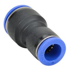
NITRA pneumatic push-to-connect fitting, union straight reducer, thermoplastic (PBT) body, (1) 16mm push-to-connect to (1) 12mm push-to-connect. Package of 5.
