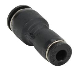
NITRA pneumatic push-to-connect fitting, union straight reducer, thermoplastic (PBT) body, 1/4in tube to 5/32in (4mm) tube connection(s). Package of 5.
