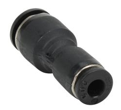
NITRA pneumatic push-to-connect fitting, union straight reducer, thermoplastic (PBT) body, (1) 1/4in push-to-connect to (1) 5/32in (4mm) push-to-connect. Package of 5.
