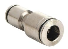
NITRA pneumatic push-to-connect fitting, union straight reducer, nickel-plated brass body, (1) 1/4in push-to-connect to (1) 5/32in (4mm) push-to-connect. Package of 5.
