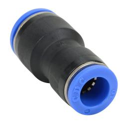
NITRA pneumatic push-to-connect fitting, union straight reducer, thermoplastic (PBT) body, (1) 12mm push-to-connect to (1) 10mm push-to-connect. Package of 5.
