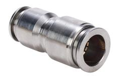
NITRA pneumatic push-to-connect fitting, union straight reducer, 316 stainless steel body, (1) 1/2in push-to-connect to (1) 3/8in push-to-connect.
