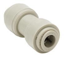
HydroMode potable water push-to-connect fitting, union straight reducer, acetal body, (1) 1/2in tube to (1) 3/8in tube connection(s), NSF/ANSI 61. Package of 5.
