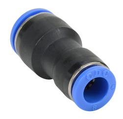
NITRA pneumatic push-to-connect fitting, union straight reducer, thermoplastic (PBT) body, 10mm tube to 5/16in (8mm) tube connection(s). Package of 5.
