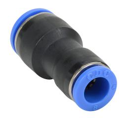
NITRA pneumatic push-to-connect fitting, union straight reducer, thermoplastic (PBT) body, (1) 10mm push-to-connect to (1) 5/16in (8mm) push-to-connect. Package of 5.
