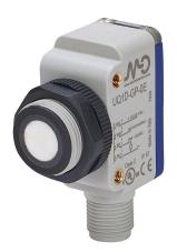
Micro Detectors ultrasonic proximity sensor, rectangular,  $53 \times 20 \times 38$ mm, polybutylene terephthalate housing, PNP, N.O./N.C. selectable output, 80-1200mm sensing distance, 3 Hz switching frequency, IP67, 4-pin M12 quick-disconnect.
