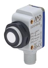
Micro Detectors ultrasonic proximity sensor, rectangular,  $53 \times 20 \times 38$ mm, polybutylene terephthalate housing, NPN, N.O./N.C. selectable output, 80-1200mm sensing distance, 3 Hz switching frequency, IP67, 4-pin M12 quick-disconnect.
