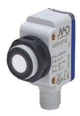
Micro Detectors ultrasonic proximity sensor, rectangular,  $53 \times 20 \times 38$ mm, polybutylene terephthalate housing, PNP, 0-10 VDC analog output, N.O./N.C. selectable output, 80-1200mm sensing distance, 3 Hz switching frequency, IP67, 4-pin M12 quick-disconnect.
