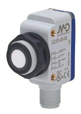
Micro Detectors ultrasonic proximity sensor, rectangular,  $53 \times 20 \times 38$ mm, polybutylene terephthalate housing, PNP, 4-20 mA analog output, N.O./N.C. selectable output, 80-1200mm sensing distance, 3 Hz switching frequency, IP67, 4-pin M12 quick-disconnect.
