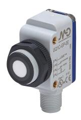
Micro Detectors ultrasonic proximity sensor, rectangular,  $53 \times 20 \times 38$ mm, polybutylene terephthalate housing, PNP, N.O./N.C. selectable output, 60-800mm sensing distance, 5 Hz switching frequency, IP67, 4-pin M12 quick-disconnect.
