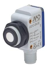
Micro Detectors ultrasonic proximity sensor, rectangular, 53 x 20 x 38mm, polybutylene terephthalate housing, NPN, N.O./N.C. selectable output, 60-800mm sensing distance, 5 Hz switching frequency, IP67, 4-pin M12 quick-disconnect.
