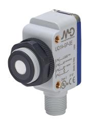
Micro Detectors ultrasonic proximity sensor, rectangular,  $53 \times 20 \times 38$ mm, polybutylene terephthalate housing, PNP, N.O./N.C. selectable output, 40-300mm sensing distance, 8 Hz switching frequency, IP67, 4-pin M12 quick-disconnect.
