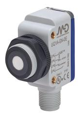
Micro Detectors ultrasonic proximity sensor, rectangular, 53 x 20 x 38mm, polybutylene terephthalate housing, NPN, N.O./N.C. selectable output, 40-300mm sensing distance, 8 Hz switching frequency, IP67, 4-pin M12 quick-disconnect.
