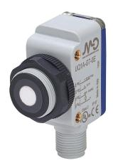
Micro Detectors ultrasonic proximity sensor, rectangular,  $53 \times 20 \times 38$ mm, polybutylene terephthalate housing, PNP, 0-10 VDC analog output, N.O./N.C. selectable output, 40-300mm sensing distance, 8 Hz switching frequency, IP67, 4-pin M12 quick-disconnect.
