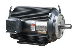
U.S. MOTORS ACCU-Torq premium efficiency AC induction motor, high-performance inverter duty, 7-1/2hp, 3-phase, 230/460 VAC, 1200rpm, TENV, NEMA 254TC frame, aluminum, C-face/rigid base mount.
