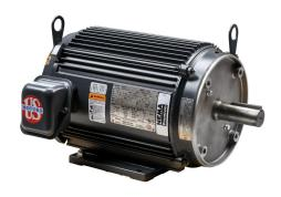
U.S. MOTORS ACCU-Torq premium efficiency AC induction motor, high-performance inverter duty, 7-1/2hp, 3-phase, 230/460 VAC, 1800rpm, TENV, NEMA 213TC frame, aluminum, C-face/rigid base mount.
