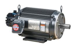
U.S. MOTORS ACCU-Torq premium efficiency AC induction motor, high-performance inverter duty, 7-1/2hp, 3-phase, 230/460 VAC, 1800rpm, TENV, NEMA 213TC frame, aluminum, C-face/rigid base mount. Avtron HS35A encoder included.
