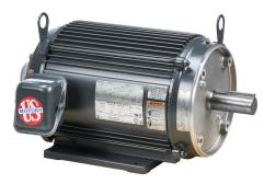
U.S. MOTORS ACCU-Torq premium efficiency AC induction motor, high-performance inverter duty, 5hp, 3-phase, 230/460 VAC, 1200rpm, TENV, NEMA 215TC frame, aluminum, C-face/rigid base mount.
