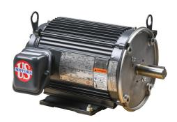
U.S. MOTORS ACCU-Torq premium efficiency AC induction motor, high-performance inverter duty, 5hp, 3-phase, 230/460 VAC, 1800rpm, TENV, NEMA 184TC frame, aluminum, C-face/rigid base mount.
