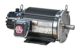
U.S. MOTORS ACCU-Torq premium efficiency AC induction motor, high-performance inverter duty, 5hp, 3-phase, 230/460 VAC, 1800rpm, TENV, NEMA 184TC frame, aluminum, C-face/rigid base mount. Avtron HS35A encoder included.
