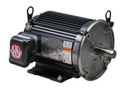
U.S. MOTORS ACCU-Torq high efficiency AC induction motor, high-performance inverter duty, 3hp, 3-phase, 230/460 VAC, 1800rpm, TENV, NEMA 182TC frame, aluminum, C-face/rigid base mount.
