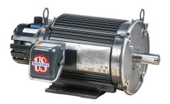
U.S. MOTORS ACCU-Torq high efficiency AC induction motor, high-performance inverter duty, 3hp, 3-phase, 230/460 VAC, 1800rpm, TENV, NEMA 182TC frame, aluminum, C-face/rigid base mount. Avtron HS35A encoder included.
