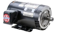
U.S. MOTORS ACCU-Torq premium efficiency AC induction motor, high-performance inverter duty, 1-1/2hp, 3-phase, 230/460 VAC, 1800rpm, TENV, NEMA 145TC frame, rolled steel, C-face/rigid base mount.
