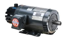
U.S. MOTORS ACCU-Torq premium efficiency AC induction motor, high-performance inverter duty, 1-1/2hp, 3-phase, 230/460 VAC, 1800rpm, TENV, NEMA 145TC frame, rolled steel, C-face/rigid base mount. Avtron HS35A encoder included.
