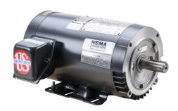
U.S. MOTORS ACCU-Torq premium efficiency AC induction motor, high-performance inverter duty, 2hp, 3-phase, 230/460 VAC, 1800rpm, TENV, NEMA 145TC frame, rolled steel, C-face/rigid base mount.
