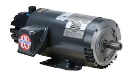
U.S. MOTORS ACCU-Torq premium efficiency AC induction motor, high-performance inverter duty, 2hp, 3-phase, 230/460 VAC, 1800rpm, TENV, NEMA 145TC frame, rolled steel, C-face/rigid base mount. Avtron HS35A encoder included.
