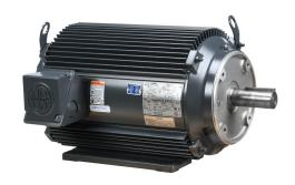
U.S. MOTORS ACCU-Torq premium efficiency AC induction motor, high-performance inverter duty, 20hp, 3-phase, 230/460 VAC, 1800rpm, TENV, NEMA 256TC frame, aluminum, C-face/rigid base mount.
