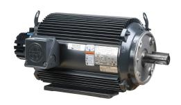
U.S. MOTORS ACCU-Torq premium efficiency AC induction motor, high-performance inverter duty, 20hp, 3-phase, 230/460 VAC, 1800rpm, TENV, NEMA 256TC frame, aluminum, C-face/rigid base mount. Avtron HS35A encoder included.
