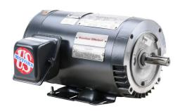
U.S. MOTORS ACCU-Torq high efficiency AC induction motor, high-performance inverter duty, 1hp, 3-phase, 230/460 VAC, 1800rpm, TENV, NEMA 56C frame, rolled steel, C-face/rigid base mount.
