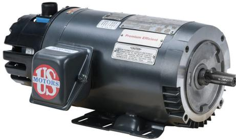
U.S. MOTORS ACCU-Torq high efficiency AC induction motor, high-performance inverter duty, 1hp, 3-phase, 230/460 VAC, 1800rpm, TENV, NEMA 56C frame, rolled steel, C-face/rigid base mount. Avtron HS35A encoder included.
