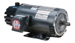
U.S. MOTORS ACCU-Torq high efficiency AC induction motor, high-performance inverter duty, 1hp, 3-phase, 230/460 VAC, 1800rpm, TENV, NEMA 56C frame, rolled steel, C-face/rigid base mount. Avtron HS35A encoder included.
