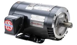
U.S. MOTORS ACCU-Torq high efficiency AC induction motor, high-performance inverter duty, 1hp, 3-phase, 230/460 VAC, 1800rpm, TENV, NEMA 143TC frame, rolled steel, C-face/rigid base mount.
