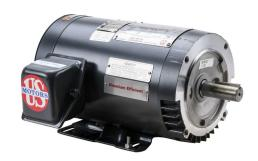
U.S. MOTORS ACCU-Torq high efficiency AC induction motor, high-performance inverter duty, 1hp, 3-phase, 230/460 VAC, 1800rpm, TENV, 143TC frame, rolled steel, C-face/rigid base mount.
