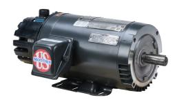
U.S. MOTORS ACCU-Torq high efficiency AC induction motor, high-performance inverter duty, 1hp, 3-phase, 230/460 VAC, 1800rpm, TENV, NEMA 143TC frame, rolled steel, C-face/rigid base mount. Avtron HS35A encoder included.
