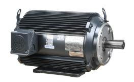
U.S. MOTORS ACCU-Torq premium efficiency AC induction motor, high-performance inverter duty, 15hp, 3-phase, 230/460 VAC, 1800rpm, TENV, NEMA 254TC frame, aluminum, C-face/rigid base mount.
