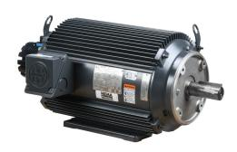
U.S. MOTORS ACCU-Torq premium efficiency AC induction motor, high-performance inverter duty, 15hp, 3-phase, 230/460 VAC, 1800rpm, TENV, NEMA 254TC frame, aluminum, C-face/rigid base mount. Avtron HS35A encoder included.
