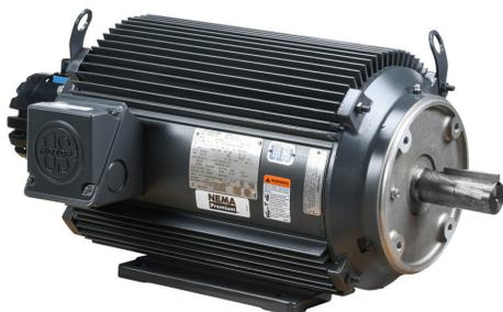
U.S. MOTORS ACCU-Torq premium efficiency AC induction motor, high-performance inverter duty, 15hp, 3-phase, 230/460 VAC, 1800rpm, TENV, NEMA 254TC frame, aluminum, C-face/rigid base mount. Avtron HS35A encoder included.
