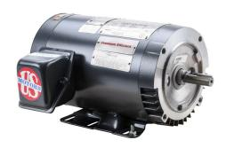
U.S. MOTORS ACCU-Torq premium efficiency AC induction motor, high-performance inverter duty, 1/4hp, 3-phase, 230/460 VAC, 1800rpm, TENV, NEMA 56C frame, rolled steel, C-face/rigid base mount.
